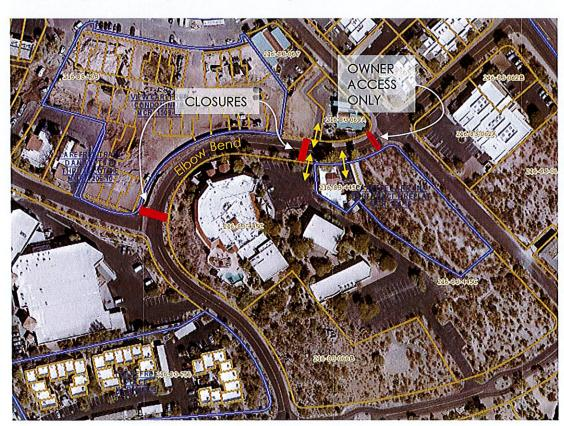
To properly repave Elbow Bend, the existing aggregate base course (ABC), a sublayer below the paving, must be removed and replaced with new ABC. This requires fine grading, compaction, and other construction procedures that necessitate additional space beyond the actual pavement installation. Staff agrees that closing this stretch of Elbow Bend will accommodate this work in an efficient and cautious manner.
