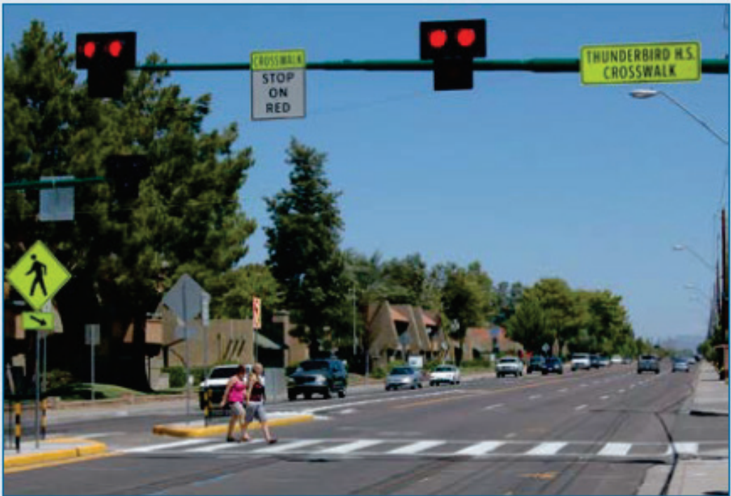
Figure 12: PHB / HAWK pedestrian crossing
